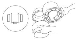
**STEP 3:** Use the flange bracket to locate where you want to mount the fan. Mark the four mounting holes.
