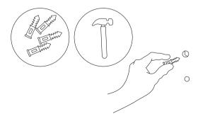
**STEP 6:** Align the fan mounting holes with the wall plate mounting location and secure the flange bracket to the mounting location with four screws or expansion screws. Make sure its airflow arrow is pointing in the direction you want it to go.
