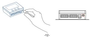
**STEP4:** Plug the adapter power cord into the controller as shown below, and finally to drive both the fan and the controller, plug the adapter power cord into an AC power outlet.
