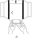
**STEP 9:** Reinstall the 2 V-shaped hooks back into the machine body so that they are connected intact.
