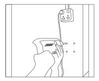
**STEP 5**: If you are installing on a concrete/brick wall, you will need to use expansion screws, expansion tubes, and fixing screws to insert into the wall mounting holes. You will need to use a hammer to make sure they are installed in place.
